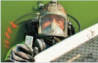
A diver retrieves temperature probes from the bottom of the Yakima River as part of monitoring for a potential fish habitat improvement project.
